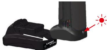
2x short flashes after battery installation — auto-test
