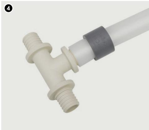
When expanding the pipes at temperatures below  $0\text{ }^\circ\text{C}$ , the expanding end of the pipe must be heated with hot water or air at temperature of  $\leq 80\text{ }^\circ\text{C}$ .
